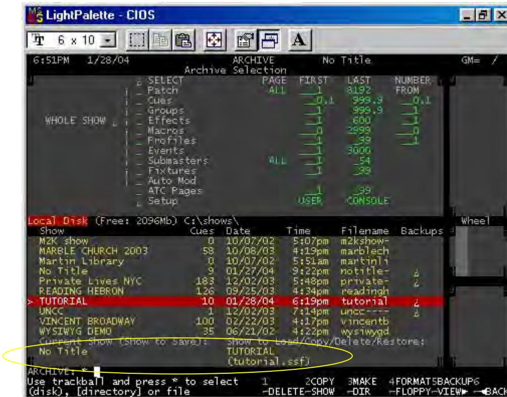
Note: Notice that the bottom of the screen shows you the Current Show (bottom left) and the Show to Load/Copy/Delete/Restore: (bottom right)
