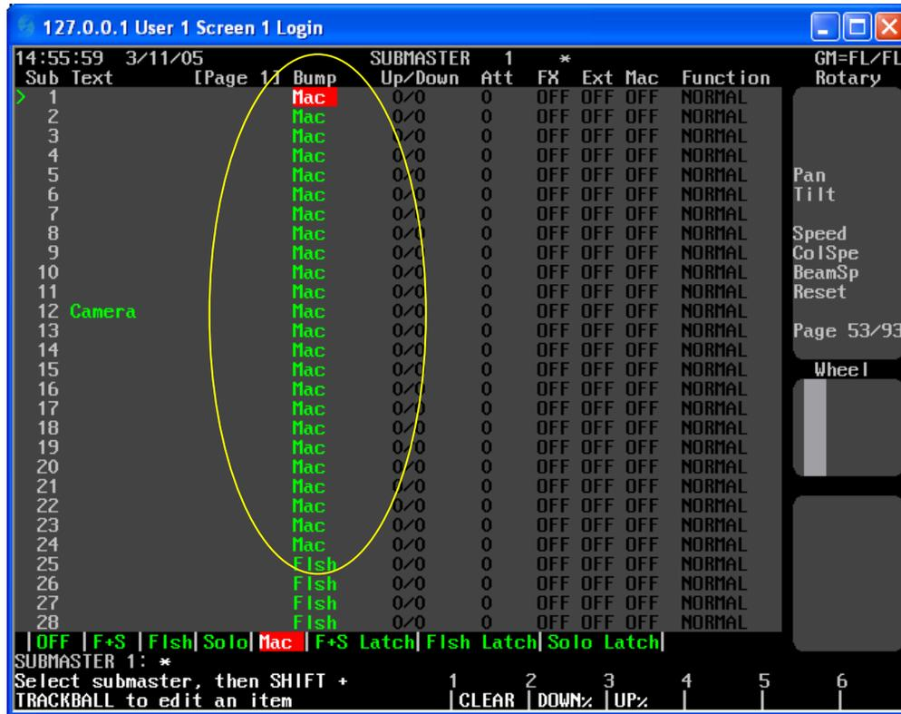
Now these subs will fire the macro equal to the sub number plus 100. So Sub 1 will fire Macro 101, Sub 24 will fire Macro 124 and so on. There is also a second page of these macros. If you hold down the *Shift* key, the bump buttons will access the sub number plus 300.
