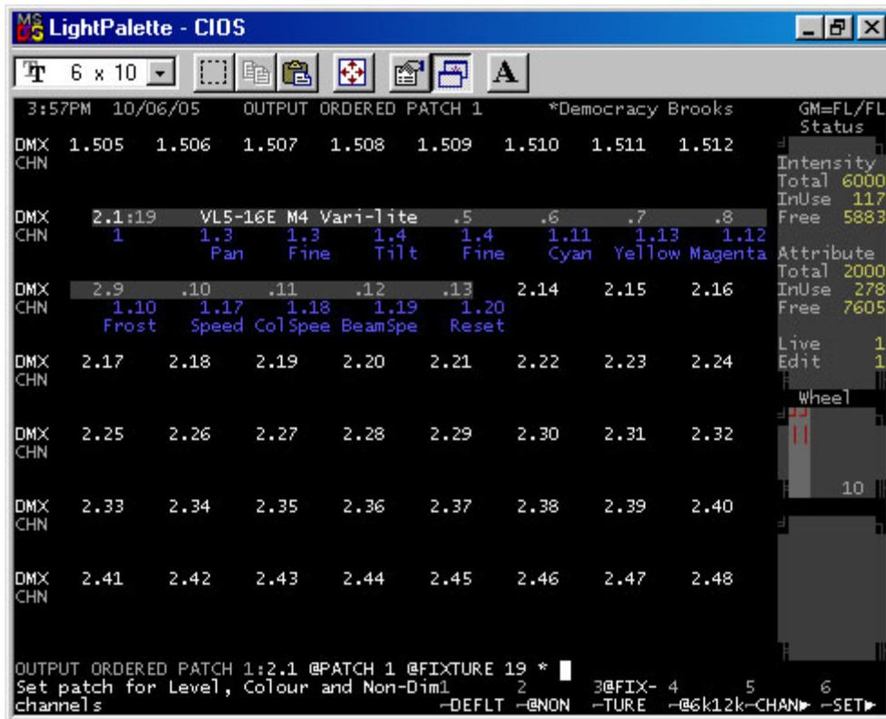
When you type in the fixture number (19 in this case) you will see the fixture name show up at the bottom of your screen. This is BEFORE you press the *Enter* key. If the number is not the correct fixture, just
