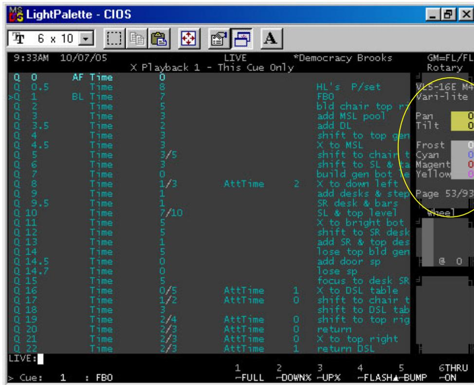
Also, if you press and hold the center teal key above the trackball and look at your softkeys, you'll see that these are ATC Pages for encoder assignments. Pressing any of these softkeys will assign that attribute grouping to the encoder wheels. The softkeys are accessing ATC Pages 51 thru 56.
