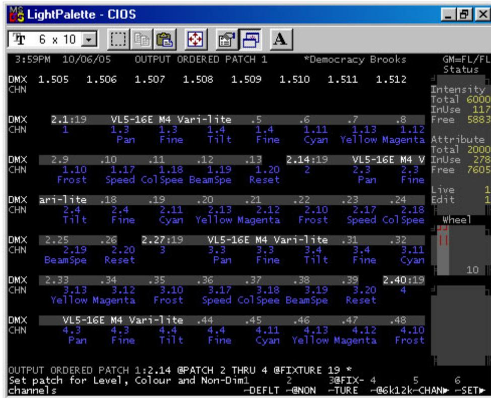
This took the next available DMX address in universe 2 and patched the VL5 to channels 2 thru 4. Notice that I didn't have to identify the starting address of every fixture. The software did that for me. This way, I can patch the show and then give the patch information to the electrician to address the fixtures.
