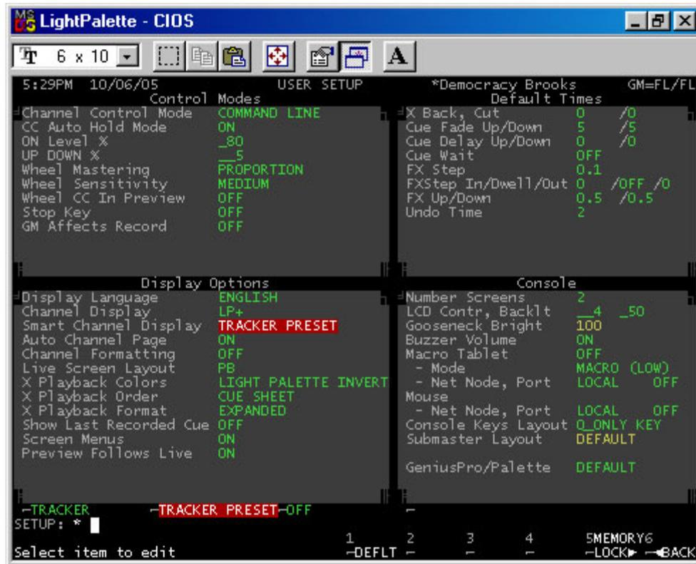
This is the way I like my User Setup screen. You don't have to copy it exactly but the important setup selection is the display option – *Smart Channel Display*. Set that to *Tracker Preset*.
