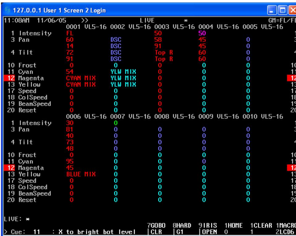
So all the channels that are in red have been selected and we know they have been adjusted by seeing the attributes that have numerical data vs showing us the text data. With the labels showing, we are seeing that the fixtures are referencing the preset focus groups. Once we adjust the information live with the trackball and encoders, the data is no longer referencing the preset focus groups. We could update
