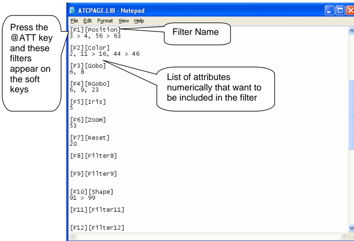
Shown here is an ATC Page that has been edited. Notice that any numerical list can be included in any filter. Just setup what is needed for speed of programming.
