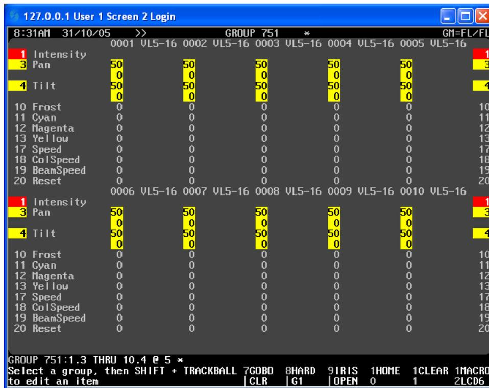
Notice that I captured the attributes that I wanted just by typing them in. The number on the left side of the point is the channel. The number on the right side of the point is the attribute number. Also notice that "THRU" worked on both sides of the point so that 1.3 thru 10.4 is actually processing 1 thru 10 but only .3 (pan) thru .4 (tilt).
