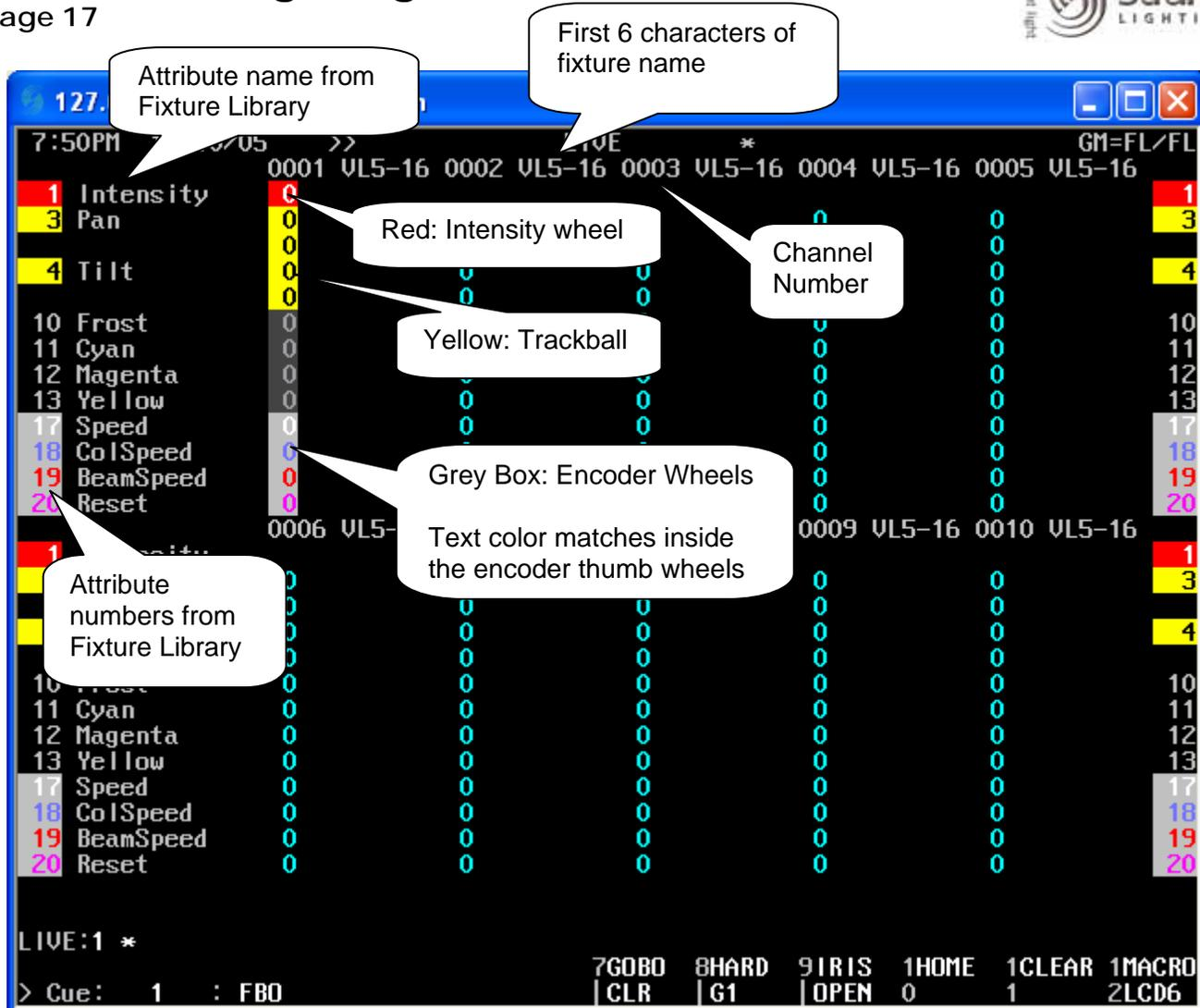
The screenshot shows a channel screen for fixture 0001 VL5-16. The interface includes a list of attributes on the left and their corresponding values on the right. Callouts explain the color coding and layout:
