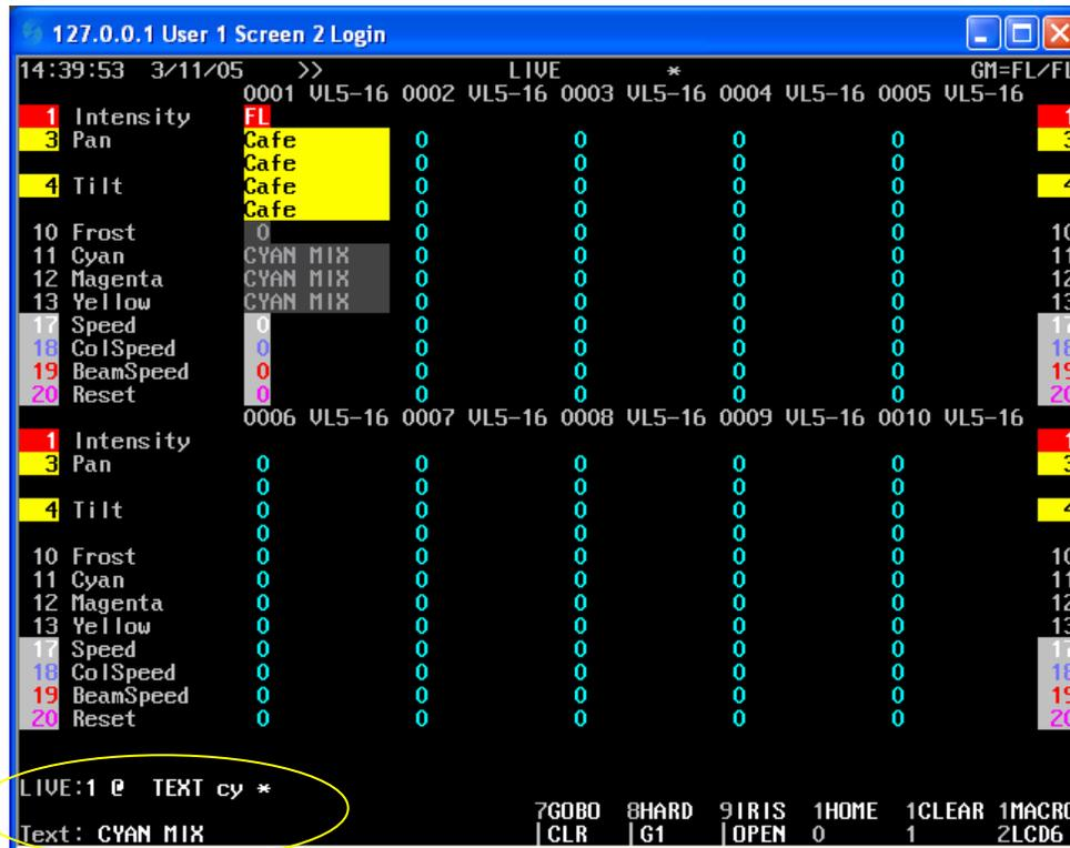
When @ TEXT is entered, the console is now looking for group label info to access the groups for you. As you enter each key, it will text match at the bottom of your screen. When the correct group label is matched, you can stop entering text and just press Enter. That's why I only typed in "CY" for Cyan Mix.
