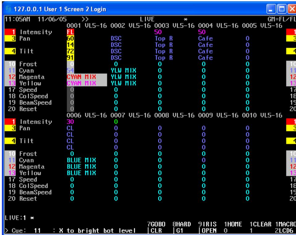
Here I've adjusted channel 1's position and the cyan wheel of the color group CYAN MIX. Now I'll adjust the other fixtures.
